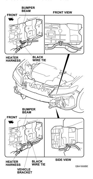
25. With the help of an assistant, route the heater harness through the front bumper opening as shown, and reinstall the front bumper.
