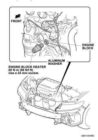
14. Plug the heater harness connector into the engine block heater. Make sure the heater harness connector is fully seated in the engine block heater.
