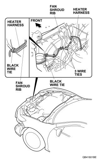
19. Secure the heater harness to the fan shroud rib with one black wire tie.
