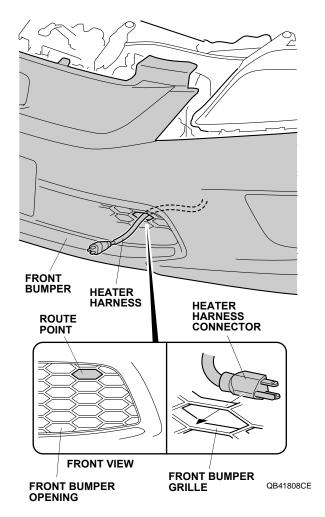
26. Secure the heater harness to the front bumper grille with one black wire tie.
