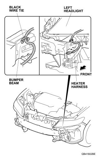
21. Route the heater harness along the vehicle harness, and secure it to the vehicle harness with two black wire ties.
