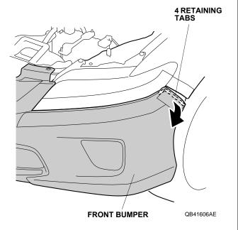
• Release the four retaining tabs on each side.
