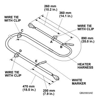
11. Using a white marker, mark the heater harness at the measurements (B) and (E).
