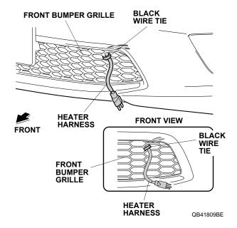
27. Install the protective cap to the front bumper grille and plug the heater harness connector into the protective cap.
